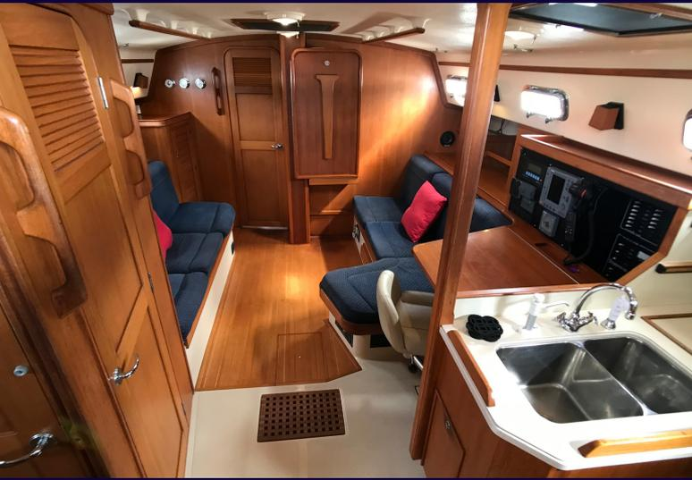
Stepping below you are amazed by the interior space. The IP420 is roomy, airy and very well ventilated with several opening ports and overhead hatches. Headroom is substantial (6'8") due to the raised coach roof. The saloon features a large double leaf table which tucks neatly away on the forward bulkhead offering a lot of interior space.
